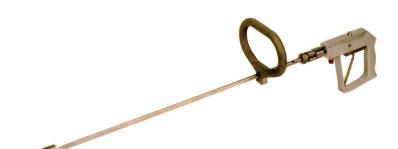
Water flow is controlled by a hand-squeeze trigger. The trigger shifts a spring-loaded plunger that normally keeps a poppet-style valve closed. When the plunger is shifted, the poppet opens and water flows to the cutting head. The Ultra Lite Lance minimizes operator fatigue during vertical and overhead applications because it is easily held in a natural horizontal position. Interchangeable extension tubes and handles are available.
